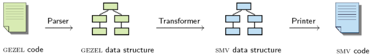
Figure 3.1: Compiling process. GEZEL code is received as input and gets stored in a data structure designed for GEZEL programs. Instead of directly producing the SMV output, the information first gets restored in a further data structure from which the SMV code is finally read and printed.
